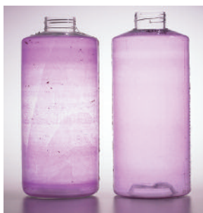
Figure 3. The roller bottle on the left was rotated too fast resulting in uneven distribution of cells to the ends of the bottle. The bottle on the right was rotated at the correct speed.
