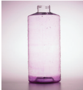
Figure 4. Most of the cells have attached to the bottom end of this bottle as a result of the roller apparatus not being level. This also can occur when bottles are stood on end for too long immediately after seeding it with cells.
