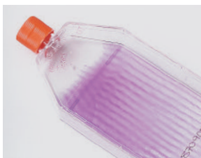
Figure 13. Vibration has caused the cells in this flask to attach in parallel rows. Moreover, the heavier cell density on the left side of this flask indicates the incubator shelf was not level.
