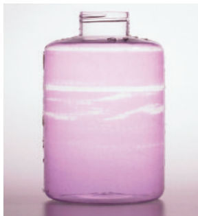
Figure 5. These clear bands were caused by debris in the medium scraping away cells as the bottle was rotated.
