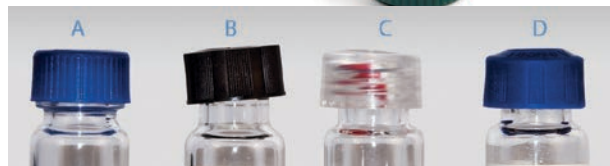
Examples of vial and closure misalignment/deformation. (A) SureStop vial self aligning cap; (B) generic vial, cap tilt; (C) generic vial, septum dislodged; and (D) generic vial, deformed top.
