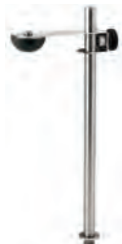
A Test tube holding device Attachment to hold one test tube safely for continuous shaking P/N 036303190
