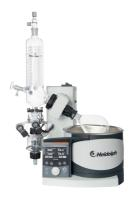
Hei-VAP Distimatic including automatic drainage of residue P/N 591-53000-00
