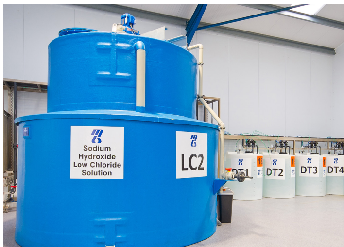
Left: Large-scale sodium hydroxide dilutions occur in these tanks Right: ISO class 8 cleanroom where all solutions are filled
