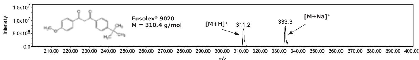
Fig. 1: Mass spectrum and structure of Eusolex® 9020, recorded at hR<sub>f</sub> value of 50 at track 5.
