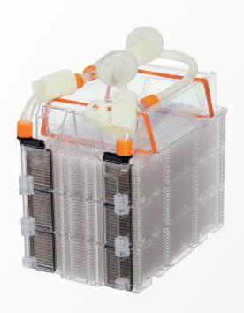
**More cells** – five times the growth surface area of a traditional vessel with a comparable footprint **Closed system** – no open fluid manipulations
