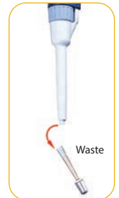
Eject to dispose of tip and FLOWMI
