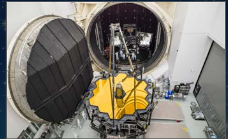
Webb Telescope Emerges from Chamber A After Cryogenic Testing
