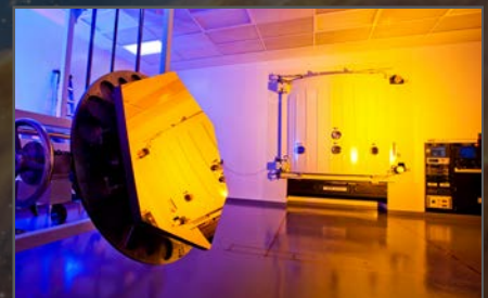
Gold-coated Engineering Design Unit (EDU) Primary Mirror Segment
