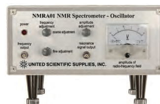
The oscillator control unit carries coarse and fine frequency adjustments and produces an RF signal of very high frequency stability.
