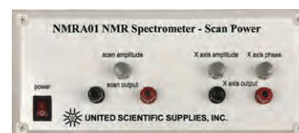
The scan control unit supplies an adjustable AC signal to the Helmholtz coils to scan the fixed magnetic field through a narrow range.
