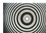
This pattern shows the full range of Zeeman-split lines emitted in the transverse direction.
