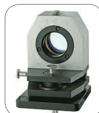
The étalon generates an interference pattern of concentric rings which is observed by a video camera.
