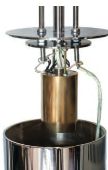
The sample heating assembly can be raised out of the oven on the telescoping support rod.
