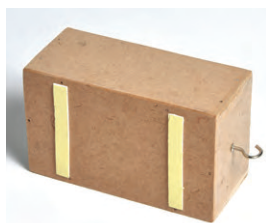
Two leather strips are attached to the bottom of the Friction Box.
