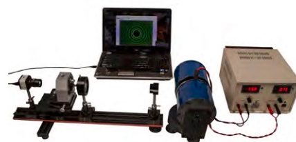
Interference patterns are observed when the Zeeman apparatus is connected to a computer.
