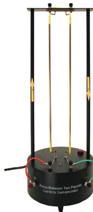
Force Between Conductors Demonstrator shown with anti-parallel connection yielding currents traveling clockwise.
