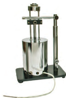
The sample oven contains a cooling fan, a massive metal block with an electric heater, three samples, and a control system sensor.
