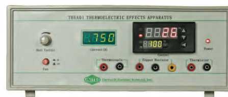
The control unit provides the heating current, connectors to the three sample devices, and the digital temperature controller.
