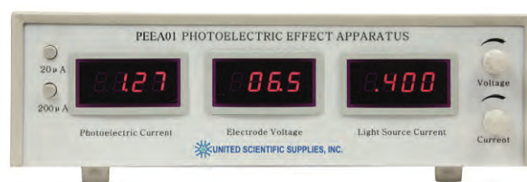
The control and measurement unit contains a highly stabilized lamp power supply adjusted by a multi-turn potentiometer.
