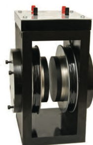
The permanent magnet generates a homogeneous field of approximately 0.5 T and is equipped with a pair of 300-turn scan coils in approximate Helmholtz arrangement.
