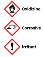
Oxidizer. Skin Sens. 1A. AcTox Oral 4. Aq Ac-Ch Tox (fish). Aq Ac-Ch Tox (Crustacea). Aq Ac-Ch Tox (Algae).
