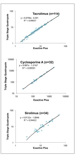
Figure 3. Correlation of results from Exactive Plus and triple-stage quadrupole instruments
