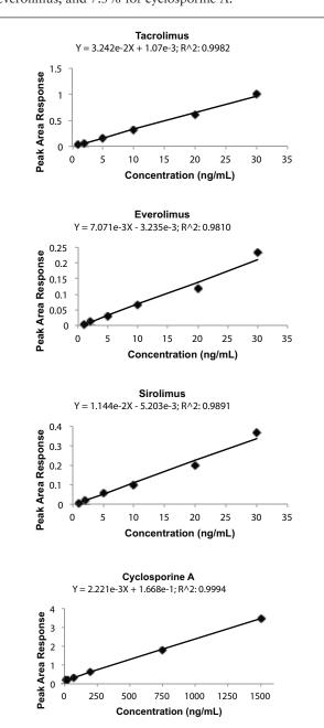
Figure 2. Representative calibration curves for immunosuppressant drugs
