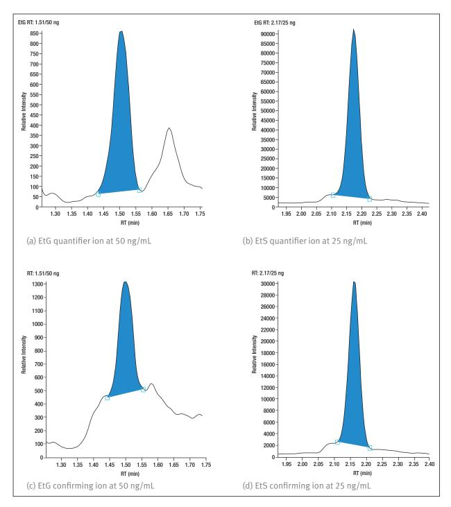
Figure 3. Representative chromatograms showing quantifier (a and b) and confirming (c and d) ions for EtG and EtS at 50 and 25 ng/mL, respectively
