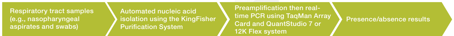
Figure 1. Workflow for detection of respiratory tract pathogens. The workflow shows extraction of total nucleic acid from respiratory tract samples using the KingFisher Purification System and MagMAX Viral/Pathogen Ultra Nucleic Acid Isolation Kit, followed by preamplification then real-time PCR analysis using the TaqMan Array Respiratory Tract Microbiota Comprehensive Card on the QuantStudio 7 or 12K Flex system. Results are provided in the form of a presence or absence call for each of 42 targets that include bacteria, RNA and DNA viruses, and fungi, and, if used, the B. atrophaeus extraction and Xeno RNA spike-in controls.
