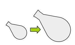
Up to 50% performance increase Doubling the evaporation flask volume can increase the performance up to
