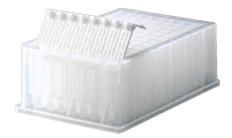
The Thermo Scientific Pierce 96-well Microdialysis Plate is an automation-compatible system for simultaneously dialyzing between 1 and 96 samples with volumes from 10 µL to 100 µL. The dialysis inserts are provided in strips of eight preloaded in a 96-well deep-well plate, but can be separated easily for use as individual dialysis devices in a standard microcentrifuge tube.
