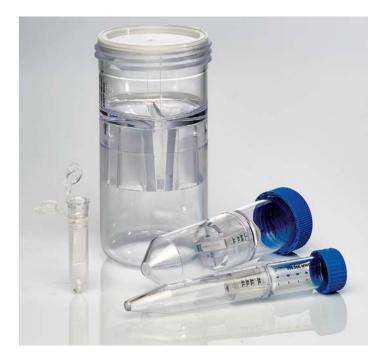
The most commonly used membranes for protein concentration devices are polyethersulfone (PES), regenerated cellulose, and cellulose triacetate (CTA). PES has a uniform surface devoid of hydrophobic or hydrophillic interactions and offers excellent protein recovery for most solutions. PES membranes exhibit
