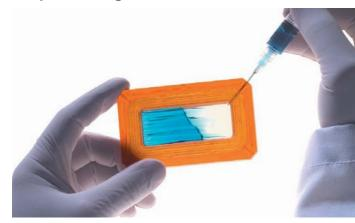
The original Thermo Scientific Slide-A-Lyzer Dialysis Cassettes facilitate rapid and effective dialysis for sample volumes from 100 µL to 30 mL. The cassette design maximizes surface area to sample volume ratio and provides excellent sample recovery. Unlike standard flat tubing, these innovative cassettes do not require knots or clips that can lead to leaking and sample loss, resulting in more complete sample recovery.
