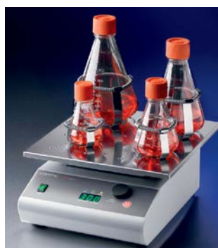
Orbital shaker with optional clamps and flasks
