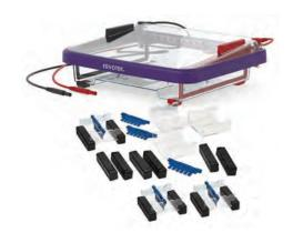
Six groups of students can load their own individual gels and six gels are run together for 30-40 minutes giving results. Eliminate cumbersome gel tray taping and pour gels quickly and easily with our innovative gel tray sealing rubber end caps.
