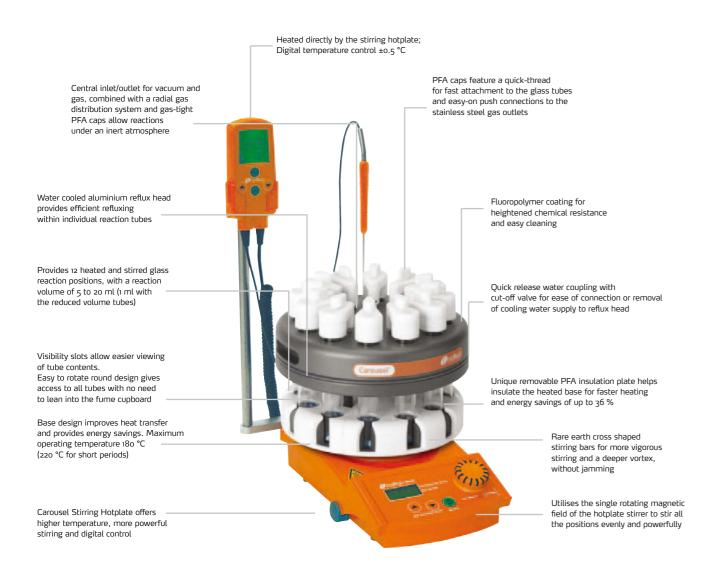
Fits on a standard hotplate stirrer so utilizing existing and readily available technology. Compact size has small bench-top footprinto easy to store
