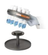
Viewing slots allow easier viewing of tube contents. Easy to rotate round design gives access to all tubes with no need to lean into the fume cupboard
