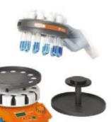
Carousel Stand is ideal for use between reactions, when changing tubes and for reactions that require rapid air cooling
