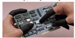
Inherently static dissipative. Not dependent on humidity. Static decay of 5000 to 0V in 0.01 second. Surface resistivity,  $2\times10^6$  ohms/sq.
