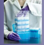
Push down with even pressure on the middle of the top insert, which will slide bottom insert into empty tray.
