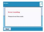
Cubis® has warning and reminder functions with a configurable action hierarchy for leveling, minimum initial weighing, and calibration | adjustment.
