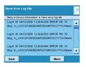
The audit trail function logs major changes to the device. For critical | validated weighing, this feature insures only accurate, reliable results.
