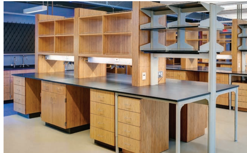
Caramelized Bamboo with edge grain island benches outfitted with electrical, plumbing and task lighting incorporated with moveable and flexible Optima™ Bench systems.
