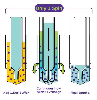
The uniquely designed interface between the exchange tube tip and the Amicon® Ultra device enables greater than 99 % buffer exchange in a single spin. Buffer exchange, as shown in this diagram, was measured by the replacement of a low-molecular weight dye (yellow) with clear buffer (black arrows); while a high-molecular weight dye (bright blue) was retained inside the Amicon® Ultra device.
