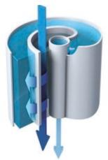
Flow-through view of an Advanced RO membrane, which is inserted into a cartridge. Tangential flow limits the risk of fouling.
