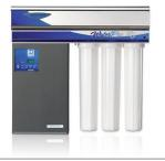
WaterPro® RO Systems. Connect to Labconco glassware washers to provide purified water for the rinse cycles. Deliver 1 L/min of reverse osmosis purified, Type III water when feedwater purity is 100 µs or better.
