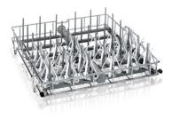
Upper Spindle Racks. 304 stainless steel. Includes 36 removable spindles, 36 adjustable height clips, 18 plastic glassware holders, 10 small spindles with clips, 36 spindle plugs, 12 spindle arm plugs and wash arm. Spindles or spindle arms may be removed and plugged to accommodate accessory inserts (sold separately). Spindle dimensions: 4.5" h x 0.25" OD. Overall dimensions: 20.8" w x 21.6" d x 6.9" h. Accommodate glassware up to 8.9" h.
