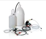
**15-352-022**—**Detergent and Acid Rinse Dispenser Kit.** Connects to any FlaskScrubber or SteamScrubber to automate liquid detergent and acid neutralizing rinse aid dispensing from bulk containers. Detergent is dispensed from one gallon plastic container and rinse aid is dispensed from one liter plastic container. Detergent and rinse aid required (not included). Shipping weight 12 lbs. (5 kg)
