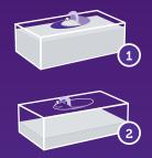
Smartpull\* dispensing incorporates 2 separate openings on the box. The first, smaller opening is used when the box is full and helps control dispensing to lessen waste from dropped gloves or multiple dispensing. When the box is half empty, the second, larger opening allows easier access to the gloves. In addition, the dispensing box also provides up to a 33% waste savings.
