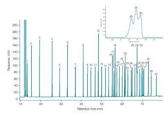
Figure 3. Chromatogram of 37 components FAME mixture (reference standard) separated on a TR-FAME GC column
