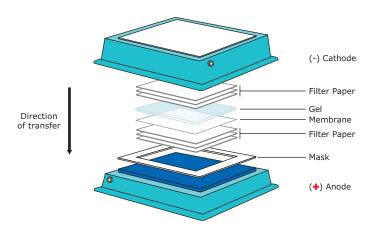
**Figure 7.**Semi-dry transfer system.
