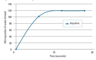
Figure 1: The speed of titration of a 1mL injection of methanol with Aqualine Electrolyte A was measured.
