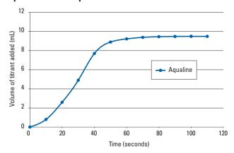
Figure 3: The titration speed of  $50\mu g$  water with Aqualine Complete 5 was recorded using an automated volumetric moisture meter.
