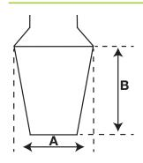
The number-pair (e.g. 29/32) describes a joint size. The first number refers to the width of the joint (A). The second number (after the slash) refers to the length of the joint (B). 29/32 therefore means that the width of the joint is 29 mm and the length of the joint is 32 mm.
