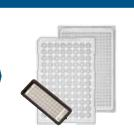
Load samples on the OpenArray PGx Panel with the OpenArray<sup>™</sup> AccuFill<sup>™</sup> System for genotyping analysis. Load samples on 384well plates for copy number analysis with TaqMan Copy Number Assays.
