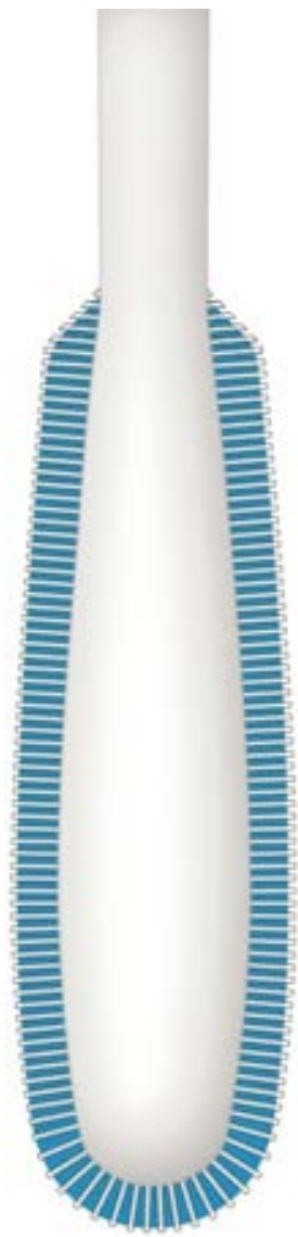
Flocked Swab Liquid sample stays close to the surface and elutes out rapidly and spontaneously
