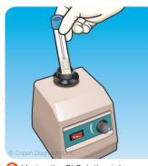
Vortex the SLSolution tube for 30 seconds at 2000-2500 RPM.
