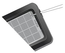
The syringe tip must be in front of the array when filling the case with immersion fluid.
