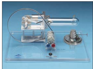
The Stirling engine includes a motor-generator and can be operated as a thermal engine, heat pump, and/or a refrigerator.
