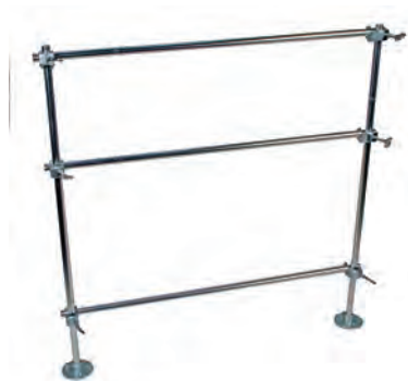
Setup with foot plates secured to a bench. Two-dimensional lattices can be assembled in units of 24" x 24" with the crossbars horizontal or vertical. The set allows construction of up to two 24" x 24" sections with one crossbar each.
