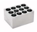
⚠ ALERTS: To avoid possible electrical hazard, DO NOT fill well or block with water or other liquids. Units are designed as a dry bath/incubator.
