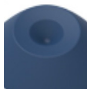
Oscillator has a shaking orbit of 4 mm
