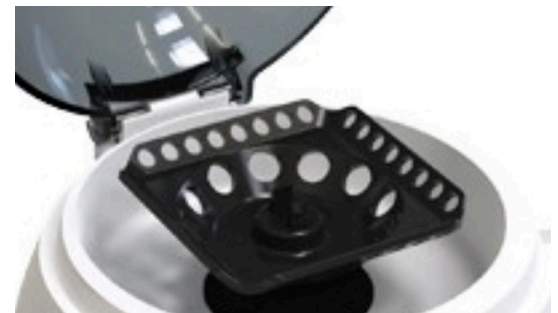
Multi-Rotor accommodates microcentrifuge tubes or PCR strips
